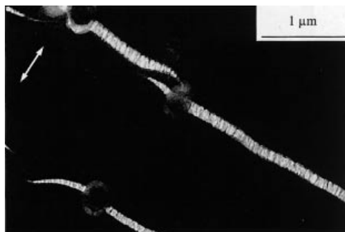
Figure 8. TEM of a thin film containing 15 wt% 3 layer particles deformed at about 1 m/s [29].
